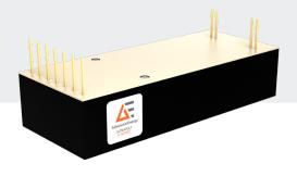
The A Series consists of miniature, PCB-mount, high voltage, regulated DC-DC converters. Designed and built utilizing state-of-the-art power-conversion topology, these units feature surface-mount technology and encapsulation techniques that provide high reliability and performance.
